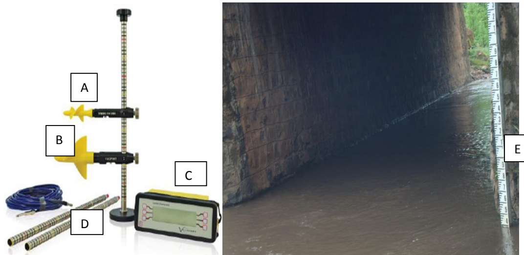
Figure 4. Current Meter model used for measuring river flow and staff gauge (E) at DR monitoring station. Photo Credit: Brihanu Zemedin (2011).
